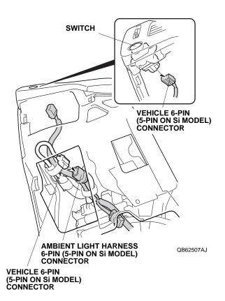
13. Plug the ambient light harness 6-pin (5-pin on Si model) connector into the switch.
