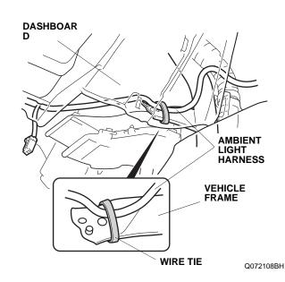
16. Inside the center lower panel opening, secure the ambient light harness to the vehicle harness with one wire tie.
