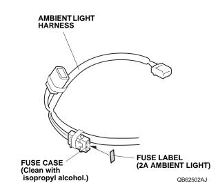
7. Attach the fuse label (2A AMBIENT LIGHT) to the ambient light harness fuse case.
