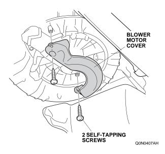
26. Using a felt-tip pen, mark the blower motor cover at the location shown.
