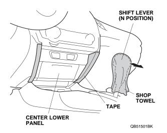
5. Remove the center lower panel (two self-tapping screws, four clips, and unplug the vehicle connectors, if equipped).
